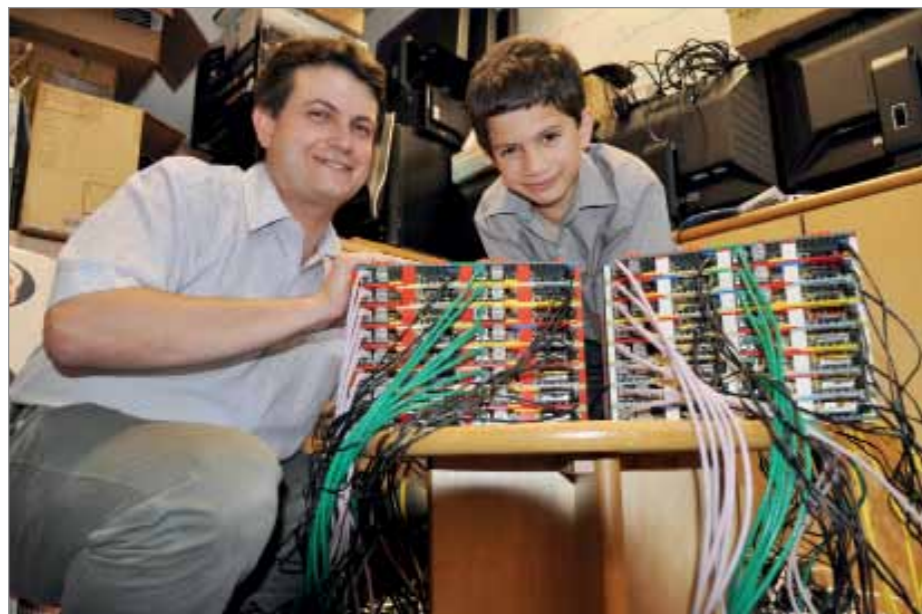
Professor Cox and his son with a cluster of Pis that link together to form a supercomputer
