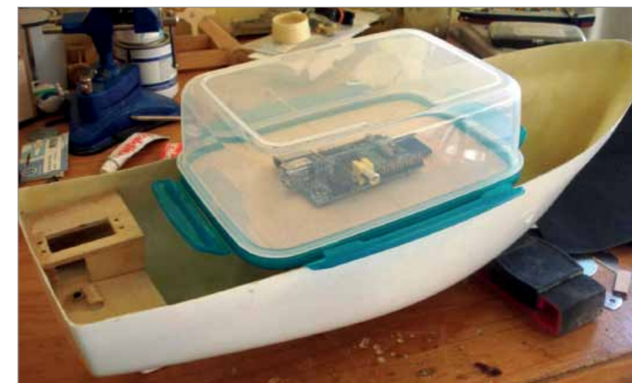
It’s still in the early stages, but Greg Holloway is hoping to develop his FishPi into an autonomous marine surface vehicle, able to perform tasks such as environmental monitoring
